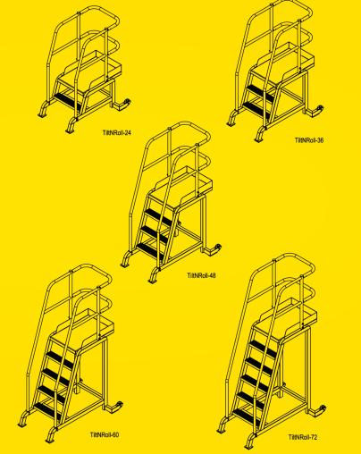
The TR Series is available in sizes ranging from 1 to 5 steps. Use the chart below to determine specifications for each size.
