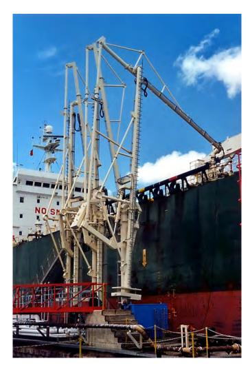
The B0030 marine loading arm is preferred when loading / unloading sea-going tanker ships and its capability has been proven with many years of trouble free operation worldwide.
